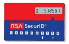
With a PINPad hardware token, the user enters the PIN on the PIN pad and then enters the resulting passcode into the RSA SecurID protected resource. With PINPad software tokens, the user enters the PIN into the software token app to generate a passcode. The user then enters the passcode into the RSA SecurID protected resource.
